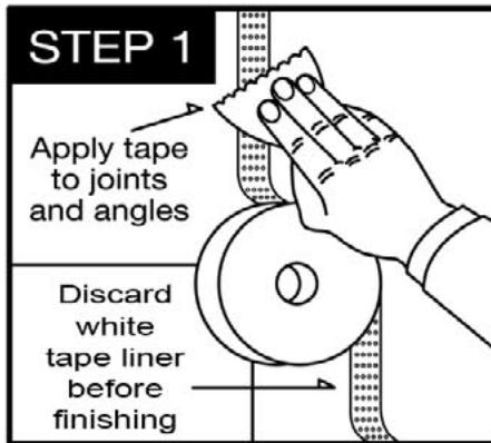
**Step 1** Apply FINISHING tape to all joints and angles of clean and dry gypsum board. Be sure the pressure sensitive adhesive, on the white paper tape, contacts the gypsum board at all times. Remove and discard the white tape protective liner. The white tape protective liner should be facing you during the application of the tape.
