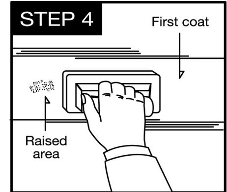
**Step 4 Allow joint compound to dry** When the joint compound is dry, remove any imperfections with a knife or sand paper. Perform normal sanding and touch-up procedures as necessary.
