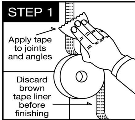
**Step 1** Apply FINISHING tape to all joints and angles of clean and dry gypsum board. Be sure the pressure sensitive adhesive, on the white paper tape, contacts the gypsum board at all times. Remove and discard the brown tape protective liner. The brown tape protective liner should be facing you during the application of the tape.
